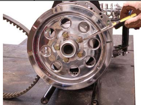
Step 16: Install the pulley on the unit using the lock ring. We also recommend Loctite.
