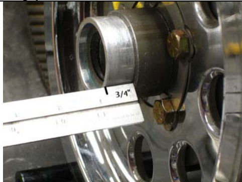
Step 17: There is a bearing spacer included with the unit. Because Harley globally sources these pulleys, we have no way of knowing how thick your pulley is. You have to measure the distance to the end. It should be 3/4 of an inch.
